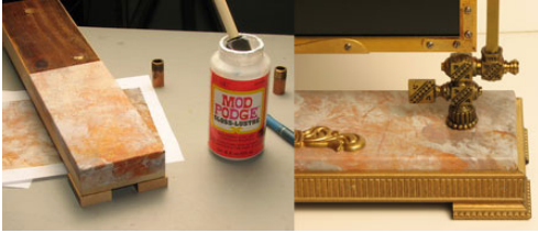
Figure 7. Monitor Base Construction: Mod Podge to affix marble pattern paper (left) and the finished base (right)
