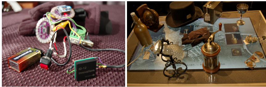
Fig. 1. Left: The components of the glove: Arduino Lilypads, XBee radio & RFID reader, Right: The 10 tagged objects on tabletop
